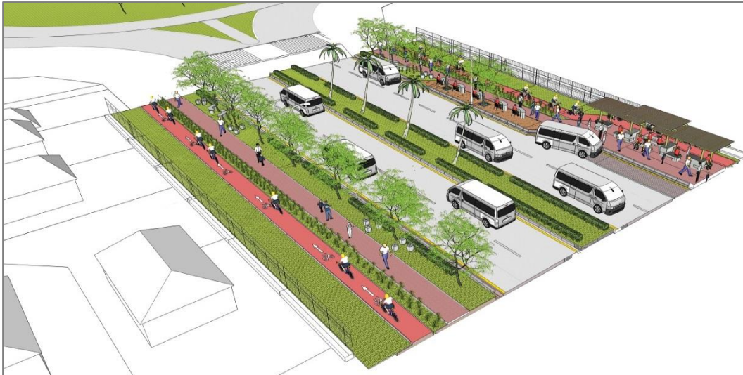
Figure 3.6: Example of a Road Cross-section with dedicated NMT
